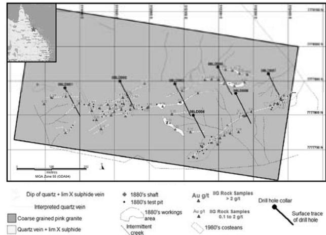
Figure 2: Conceptual Model of Lionel Diggings high grade gold mineralisation shoot/s (Not to scale)
